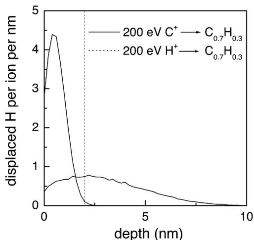
Fig. 3. TRIM calculation for the displacement of bonded hydrogen atoms per nm and ion in a  $C_{0.7}H_{0.3}$  film for incident hydrogen and carbon ions with a kinetic energy of 200 eV. The vertical dotted line indicates the penetration depth of incident thermal hydrogen atoms.
