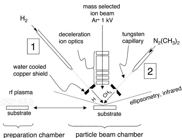
Fig. 1. Sketch of the experimental setup. A-C:H films are deposited from a r.f. discharge from methane in a preparation chamber. The samples are transferred in vacuo in the particle beam chamber equipped with two radical sources for H and CH<sub>3</sub> and a mass and energy selected ion beam.
