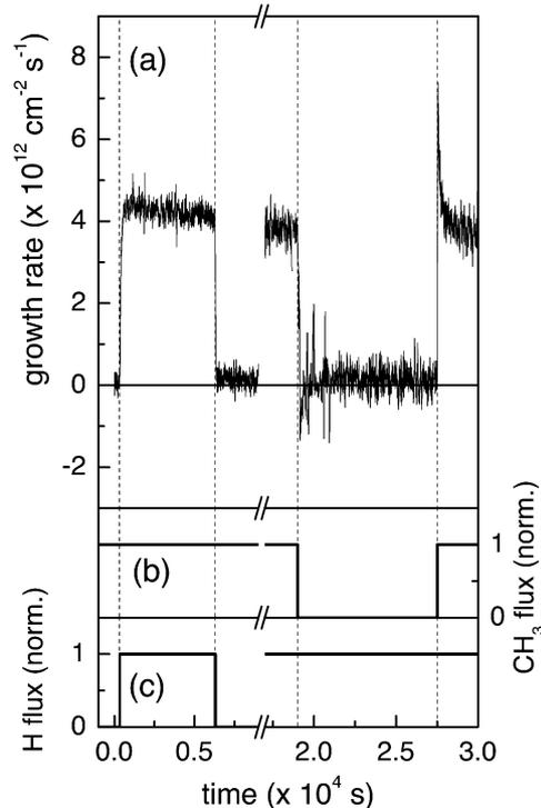
Fig. 2. (a) Variation of the growth rate during the interaction of an a-C:H film with the H and CH<sub>3</sub> radical beam at a substrate temperature of 320 K. (b) Variation of the CH<sub>3</sub> flux normalized to  $3 \times 10^{14} \text{ cm}^{-2} \text{ s}^{-1}$ . (c) Variation of the H flux normalized to  $1.4 \times 10^{15} \text{ cm}^{-2} \text{ s}^{-1}$ .
