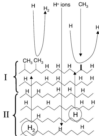
Fig. 4. Schematic of the growing film surface. I: Chemistry dominated growth zone. Incident atomic hydrogen eliminates surface bonded hydrogen via abstraction and creates chemisorption sites for incoming saturated hydrocarbon radicals. II: Ion dominated growth zone. Penetrating ions displace bonded hydrogen within the collision cascade. Displaced hydrogen might recombine to form  $H_2$  molecules or it might re-saturate dangling bonds in the film or at the physical surface.
